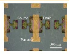
Room-temperature printed electronics are realized as a low-cost, large-area fabrication method for flexible electronic devices. Development of a  $\pi$ -junction gold nanoparticle ink enables the formation of fully printed organic thin-film transistors under atmospheric conditions at room temperature. The printed transistor devices exhibit average field-effect mobilities of 7.9 and 2.5 cm $^2$  V $^{-1}$  s $^{-1}$  on plastic and paper substrates, respectively.
