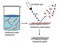
Graphene papers are prepared by irradiation of graphene oxide papers with Ar+ ion beam. Surface of the paper is chemically reduced and C/O ratios over 100 are achieved. The resulting surface is highly conductive and electrical Ohmic behavior is observed. Gases evolved during irradiation process are also analyzed.
